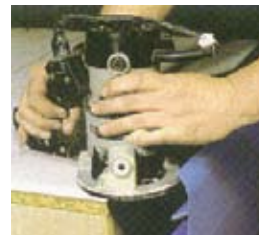
Chip deflector in the up position for use while routing.
