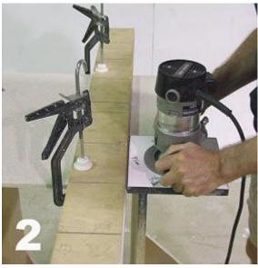
2. The square base rides along the edge 3. Place a D producing a smooth, clean edge for seaming. This base has two edges set 1/16" closer to the bit so a rough cut can be done before a finish cut without clamp so changing settings. This base is similar to our **C1-Base**.
