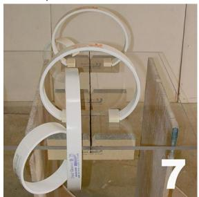
7. Stretch an orange DS8 clamp over the 8. Carefully apply the rest of the EM6 nylon seam blocks. Recheck for squeeze out. If you need to move the panels for alignment simple slide one end of the clamp in the opposite direction you want the deck to slide.
