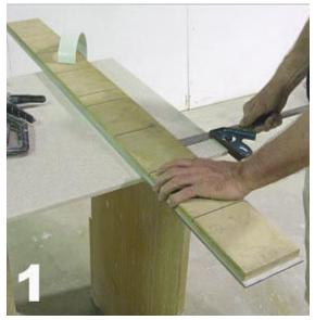
1. First you'll set a straight edge on the deck for your router to ride against. Note the deck is good side down at this point. Dani recommends using a square base on the router instead of a template guide. This method produces a smoother edge. One EM6 clamp (black) is placed at one end of the edge acting as a third hand while measuring the setback.
